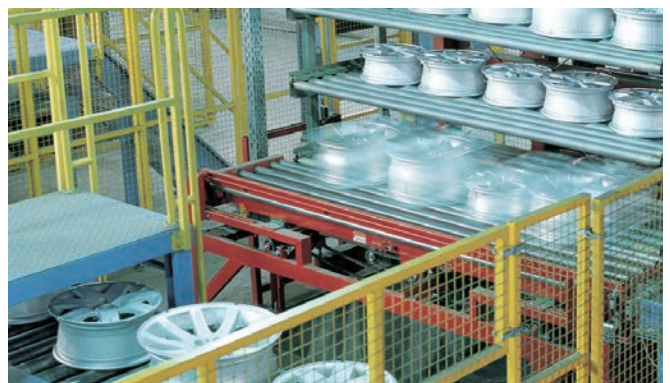
Lifting and loading device for a solution annealing furnace.
