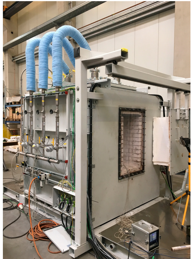
picture: Validation batch kiln for Pusher Kiln technology in the test center
