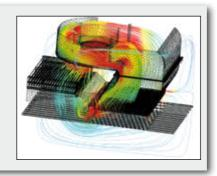
$Rough\ cooling-Identification\ of\ stalls\ above\ the\ product\ and\ constructional\ adjustment\ of\ the\ flow\ channel$
